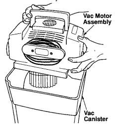
4. Turn vac canister lock into locked position.
